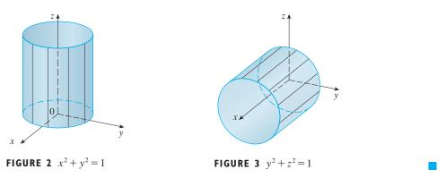
NOTE When you are dealing with surfaces, it is important to recognize that an equation like  $x^2 + y^2 = 1$  represents a cylinder and not a circle. The trace of the cylinder  $x^2 + y^2 = 1$  in the *xy*-plane is the circle with equations  $x^2 + y^2 = 1$ , z = 0.
