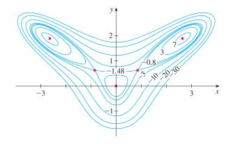
• The five critical points of the function *f* in Example 4 are shown in red in the contour map of *f* in Figure 9.
