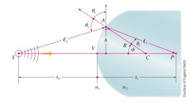
**FIGURE 8** Refraction at a spherical interface
