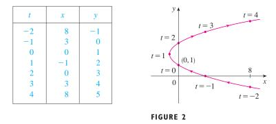
A particle whose position is given by the parametric equations moves along the curve in the direction of the arrows as t increases. Notice that the consecutive points marked on the curve appear at equal time intervals but not at equal distances. That is because the particle slows down and then speeds up as t increases.
