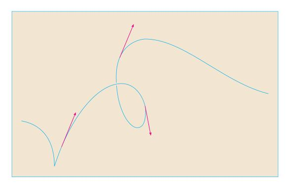
Tangent vectors show the direction in which a space curve proceeds at any point.
