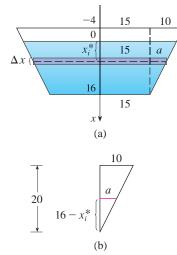
Adding these forces and taking the limit as  $n \to \infty$ , we obtain the total hydrostatic force on the dam:
