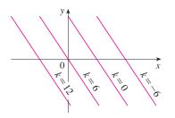
**FIGURE 15** Contour map of f(x, y) = 6 - 3x - 2y
