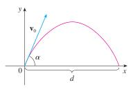
If you eliminate t from Equations 4, you will see that y is a quadratic function of x. So the path of the projectile is part of a parabola.
